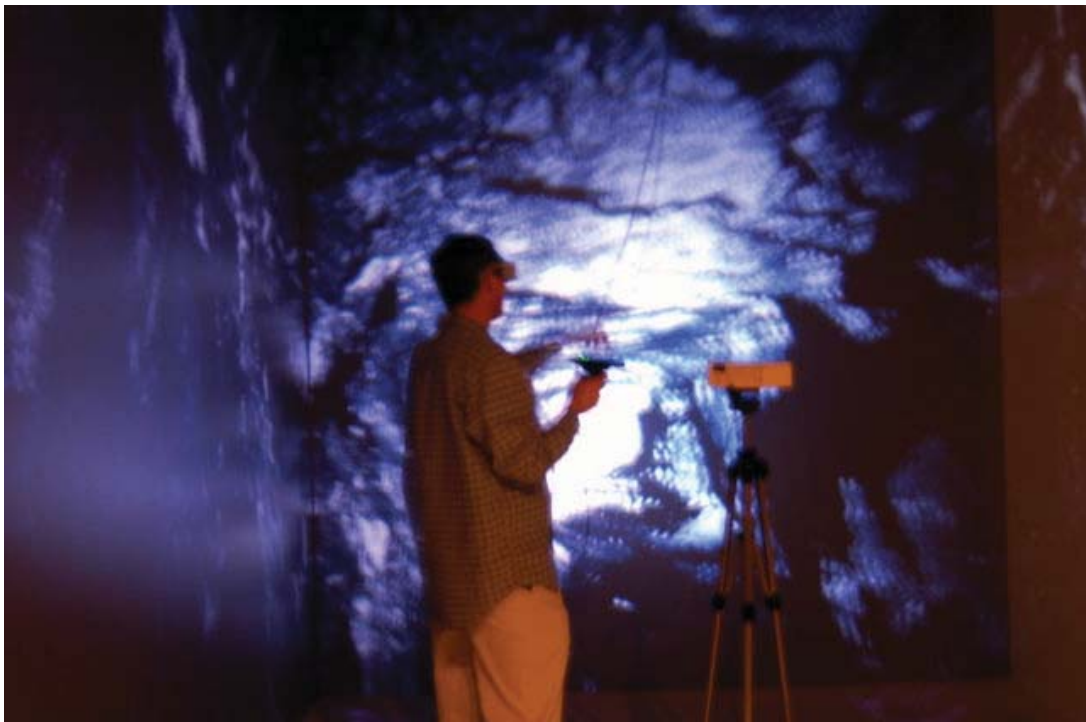
Figure 1: LIDAR point cloud data from tunnel in Eggleston, VA being viewed in a fully immersive 3d environment within VT's CAVE.
